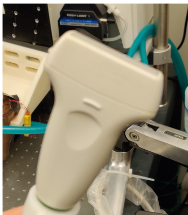
Figure 2: The Ultrasonix L14-5/38 linear array transducer used in the calibration experiment
